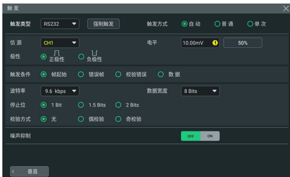
图 8.25 RS232 触发类型配置菜单
