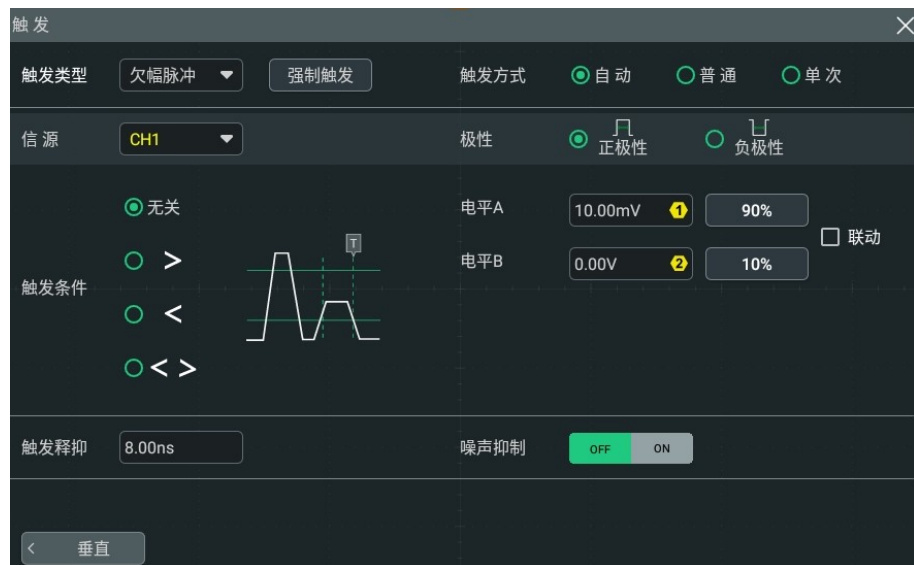
图 8.16 欠幅脉冲触发配置菜单
